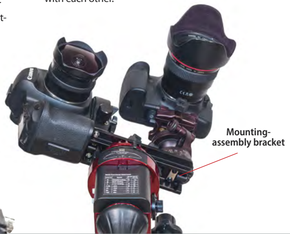
ASTRO CONFIGURATION #1 The more costly Astro Bundle includes this mounting-assembly bracket, which allows the user to attach two cameras, one in landscape orientation via a ball head and one in portrait orientation via the declination axis. Two cameras side by side in landscape orientation would collide with each other.
